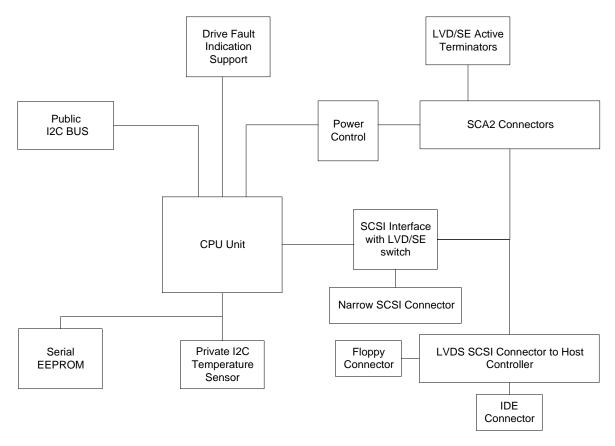
Figure 8-2: Functional Block Diagram
